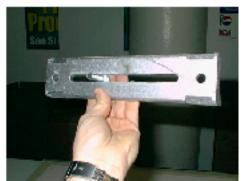
Insert stove bolt from behind through elongated slot and hold in place.
